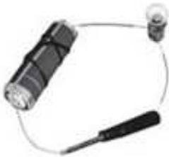
**Answer:** The bulb in the given arrangement would not glow because one of the terminals of the bulb is connected to that end of a screwdriver which is plastic. Plastic is an insulator and hence do not allow electric current to pass through it.
