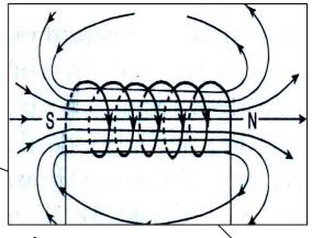
b) <u>Factors on which Magnetic Field Depends</u>: Experiments show that the magnitude of the magnetic field inside a solenoid is: directly proportional to the number of turns in the coil i.e.,  $B \propto n$ directly proportional to the strength of the current. i.e.,  $B \propto I$
