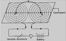
Thus, The magnetic lines of forces near each segment of wire are circular and form concentric circles with ever increasing radii as we move away from the wire, whereas the lines of force near the centre of the coil are in the form of big arcs appearing almost as straight lines.
