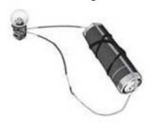
**Answer:** No, the bulb will not glow because both the wires are connected to the same terminal of the bulb.
